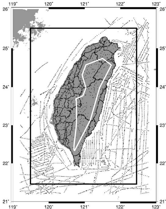
Fig. 1. Distribution of the terrestrial and marine gravity data-points in the target area (enclosed by the rectangle). The white polyhedral bounds the mountainous area (average  $H > 1200$  m), where the airborne data will be used for the gridding.
