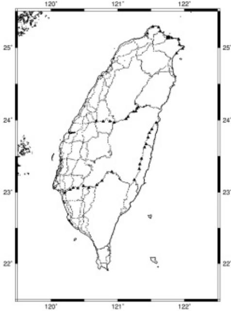
Fig. 1: Distribution of benchmarks in the first-order vertical network of Taiwan (completed in 2003). The triangles represent benchmarks where modeled and “observed” geoidal heights are compared. Square represents the origin of network at Keelung
