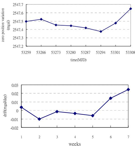
Fig. 5. (a) Variation of zero position of the Graviton EG and (b) daily drift.
