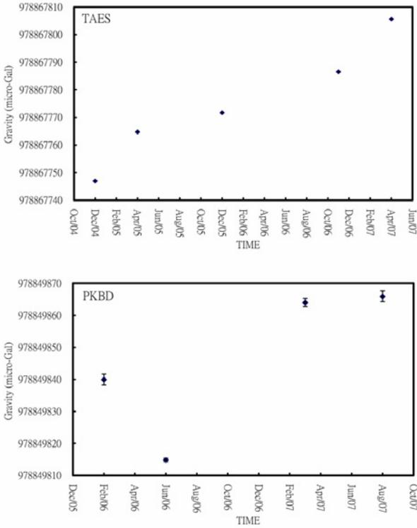
Fig. 6. Gravity values at the absolute gravity stations TAES and PKBD
