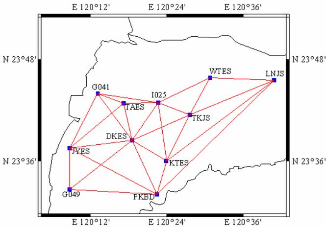
Fig. 2 Distribution of FG5 gravity stations (TAES and PKBD) and relative gravity stations for land subsidence monitoring.
