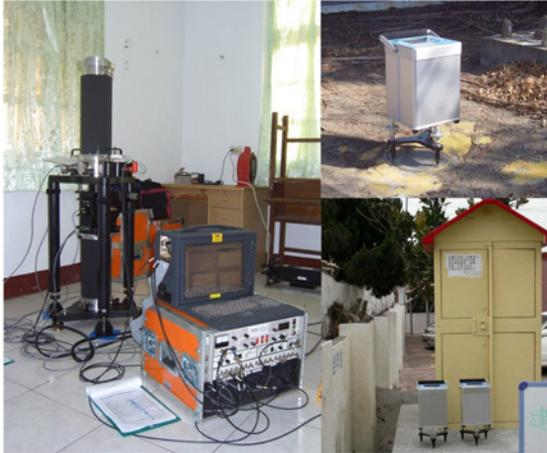
Fig. 3. (left) Measuring gravity value with a FG5 at TAES, (right) Measuring relative gravity value with CG-5 (top) near a monitoring well of ground water.
