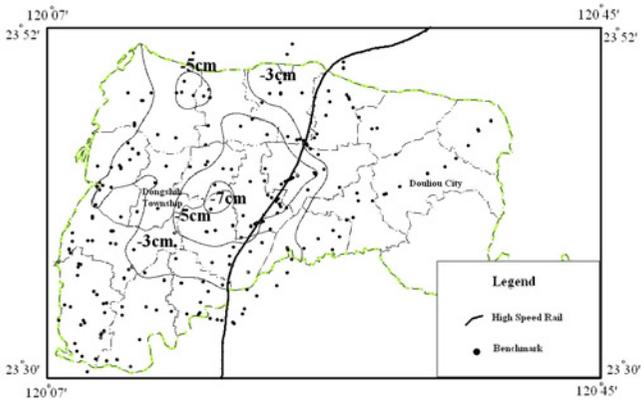
Fig. 8. Mean annual subsidence in Yunlin from precision levelling from May 2005 to August 2007.
