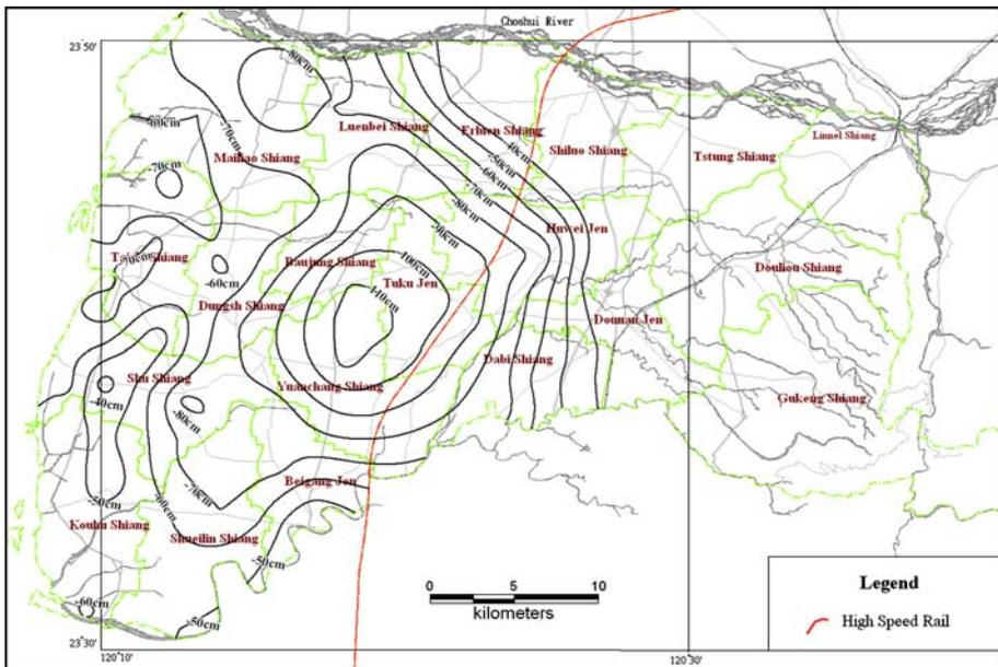
Fig. 2 Cumulative subsidence in Yunlin from 1992 to 2006
