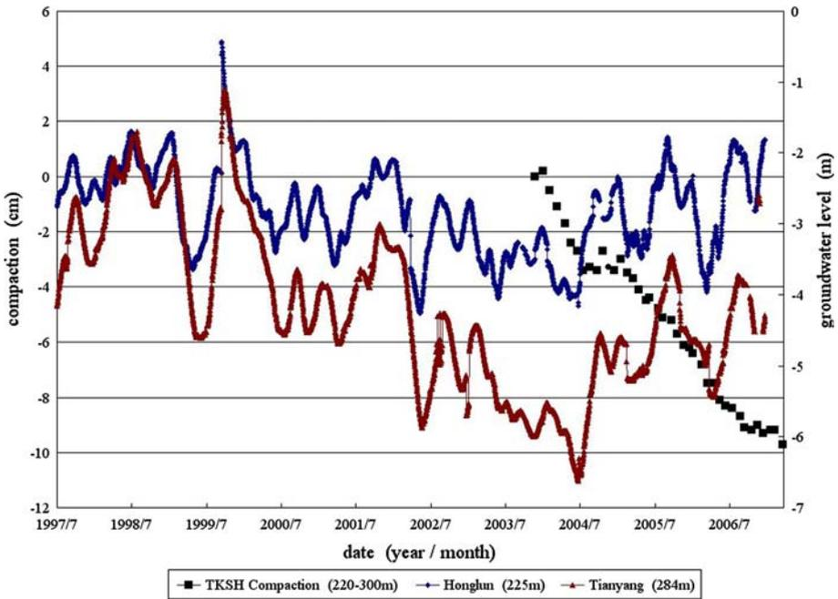
**Fig. 8** Cumulative compaction measured at depths greater than 220 m and ground water level at the TKSH monitoring well
